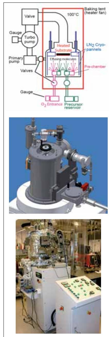
Figure 1: Schematic cross section through CBE process chamber (EPFL, top), CAD drawing of new reactor (ABCD, middle), photograph of new reactor (ABCD, bottom)
