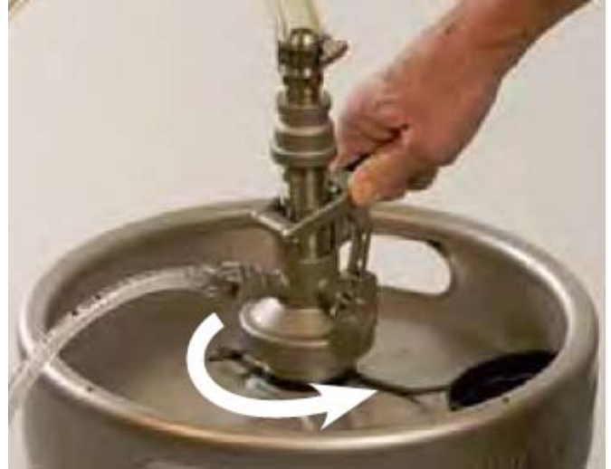
Figure 9. Removal of Coupler
