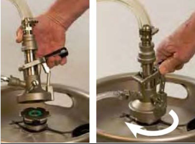
Figure 6. Rotation of Coupler
