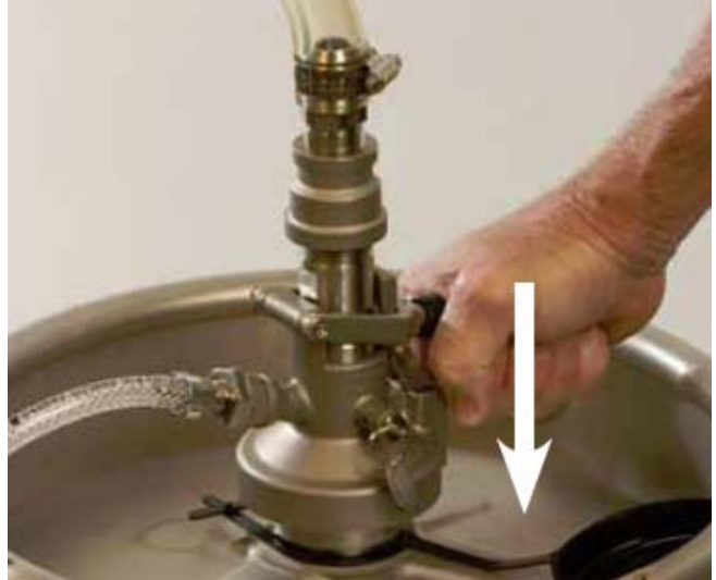
Figure 7. Engaging the coupler
