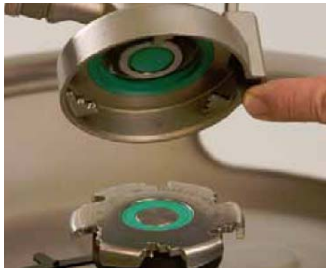
Figure 5. Alignment of the coupler notched key with extractor valve
